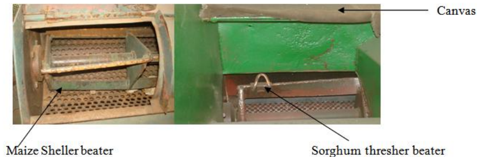
Figure 1. Beaters of maize sheller and modified sorghum thresher.
